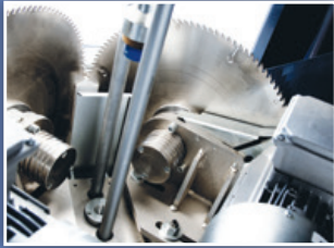
View of the pneumatic system for controlling the up and down movement of cutting saw blades
